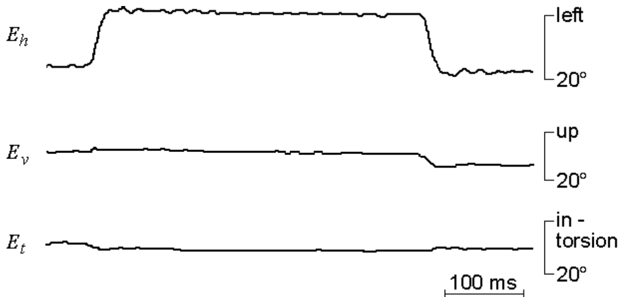
Figure 2. Example of saccades obtained in a head-restrained rat. The eye position traces E_h , E_v , and E_t correspond to the output signals A1 , A2 , and B2 of the Angle-Meter. No correction for true torsion nor for deviation from space quadrature of the dual-search coil ( \sigma = 88^\circ ).
